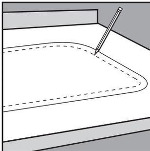
**STEP FOUR:** Measure in 3/4" and draw new lines inside the first sink outline just drawn (or taped).
